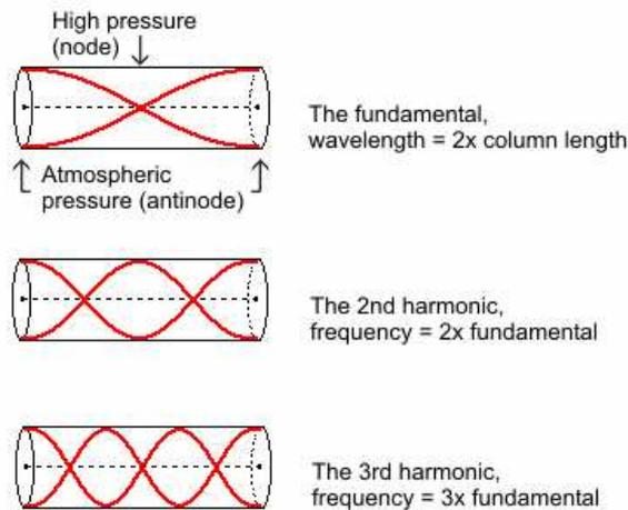
Figure 3: the Fundamental, 2<sup>nd</sup> and 3<sup>rd</sup> harmonics in a column of air open at both ends.
