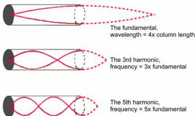
Figure 4: the Fundamental, 3<sup>rd</sup> and 5<sup>th</sup> harmonics in a column of air closed at one end.
