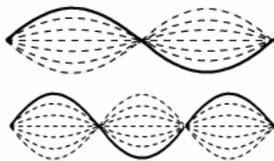
Figure 2: the 2<sup>nd</sup> and 3<sup>rd</sup> *harmonics* in a fixed string.
